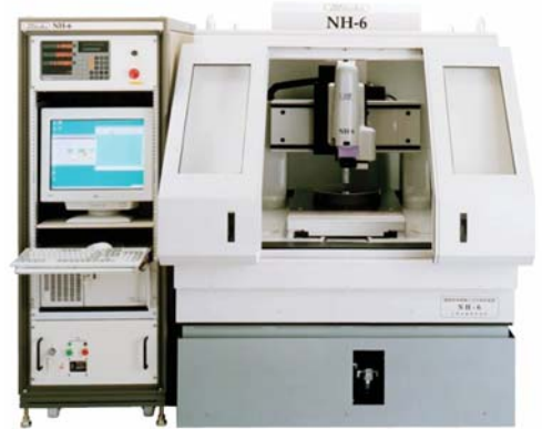
This laser-probe measurement device directly measures such instruments as liquid crystal display patterns and aspheric-surface mirrors.
